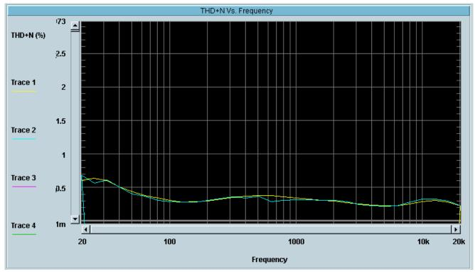
Ideally the percentage of distortion should be well below the manufacturer's specification over the entire frequency range.
