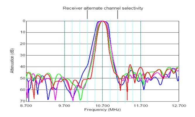
Ideally the receiver's IF amplifier selectivity should be sharply tuned to maximize sensitivity and reduce adjacent station interference, while allowing the full FM audio signal to be captured. Critically adjusting each stage of the IF allows the width and slope of the band pass filters to capture the full frequency response of the broadcast signal while limiting noise and multi-path distortion.
