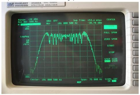
Ideally the receiver's IF amplifier selectivity should be sharply tuned to maximize sensitivity and reduce adjacent station interference, while allowing the full FM audio signal to be captured. Critically adjusting each stage of the IF allows the width and slope of the band pass filters to capture the full frequency response of the broadcast signal while limiting noise and multi-path distortion.
