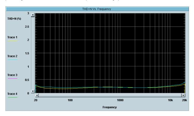
Ideally the percentage of distortion should be well below the manufacturer's specification over the entire frequency range.
